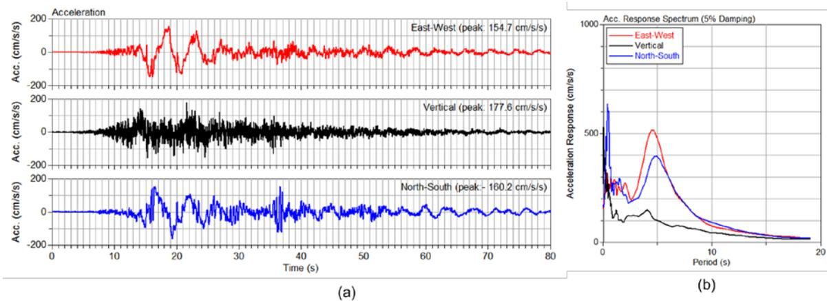
Figure 1. Ground motion recorded at Kantipur station, Kathmandu: (a) time history, (b) response spectra (5% damping).
