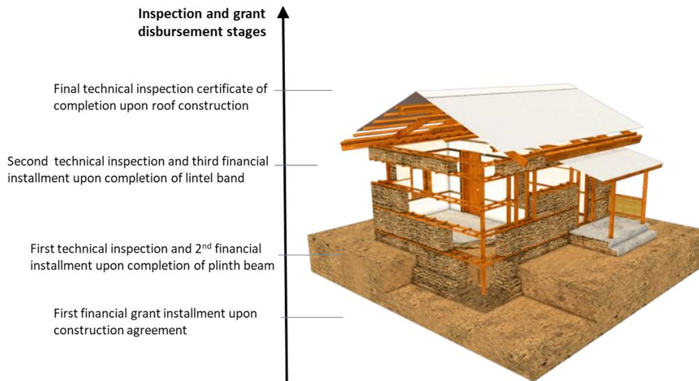
Figure 7. Schematic illustration of reconstruction inspection stages of rural houses supported by the government grant system
