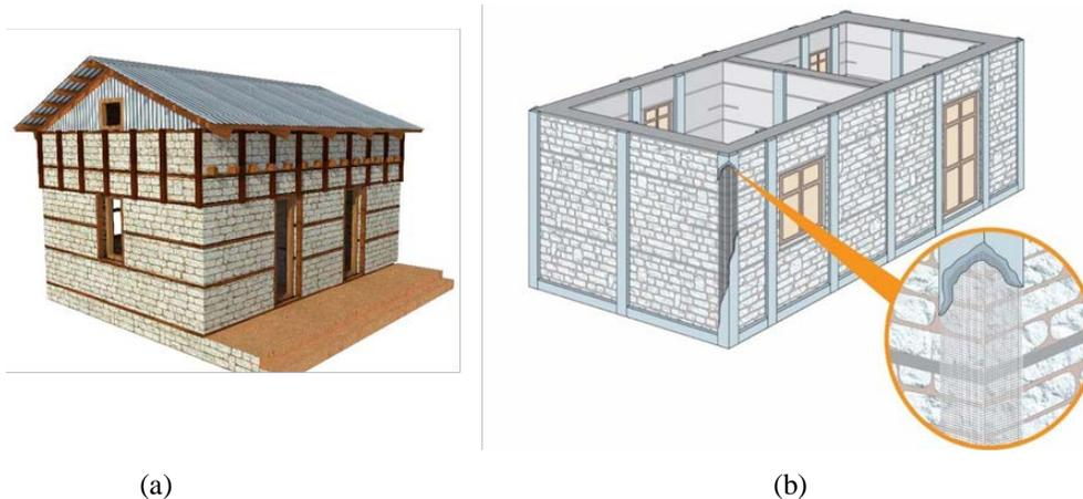
Figure 9. Vertical and horizontal reinforcement provisions for stone masonry houses: (a) using timber as the reinforcing elements (b) use of wire mesh as the reinforcement
